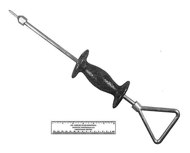
A car repair tool used to pull dents out of metal body parts, the slide hammer can be used to rip out door locks, ignition circuits, and car stereos.
